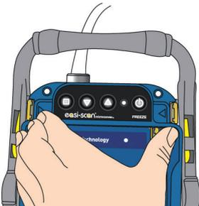
Press the Easi-Scan firmly into place. Make sure that the clips are fully engaged.
