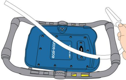
Feed the Easi-Scan probe cable through the lower handle of the Smart Display.
