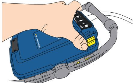
Locate the rear of the Easi-Scan under the lip at the rear of the Smart Display and press the scanner down.
